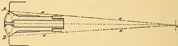
Fig. 33. Showing lines of force in clamping a chuck.
