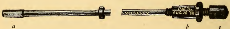
Fig. 44. Stepping Device. a —rests in chuck and should be slightly less than diameter of work. b —tightens in rear of draw-in spindle. c —turning this regulates depth of step.
