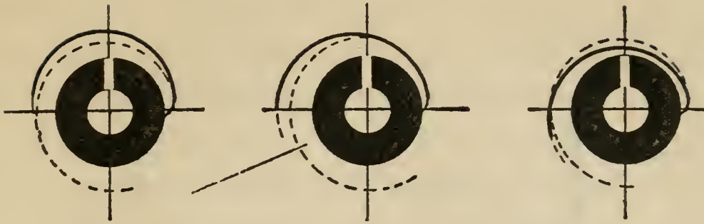
Figure 32. Dotted lines indicate manner in which the balance spring is twisted to true in the round.
