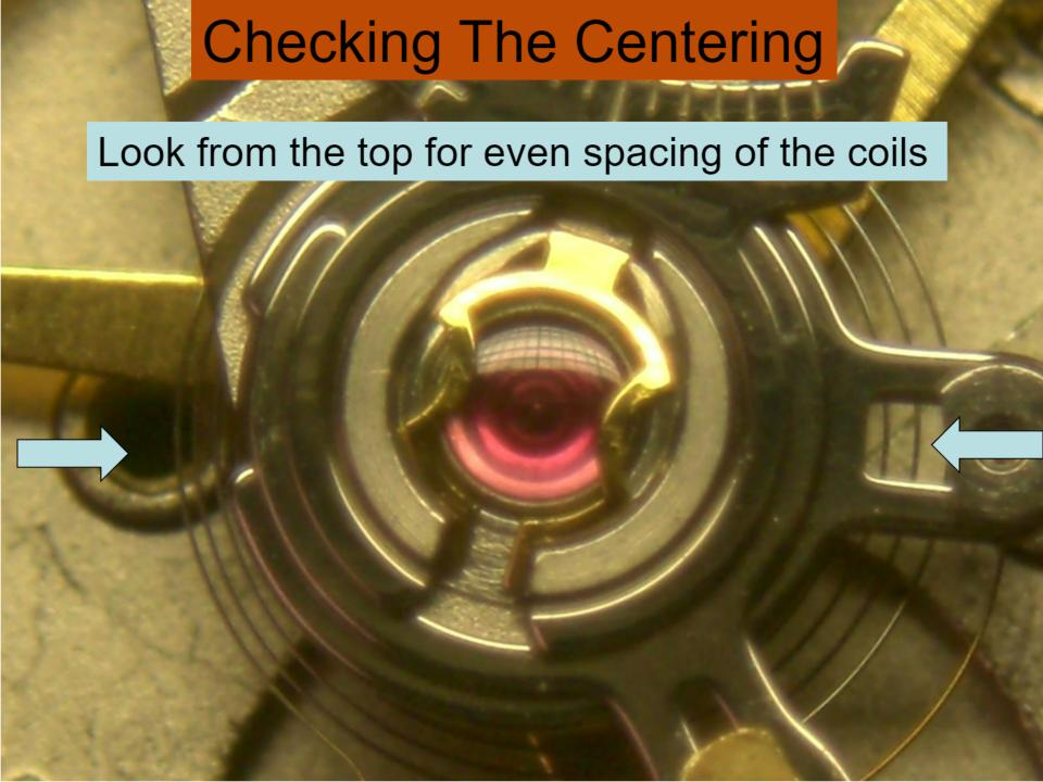
Place tool on the stud block & slightly rotate (back and forth) to center the hairspring
