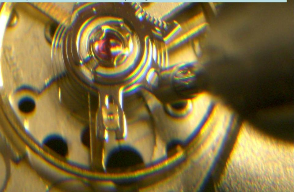
It is best to view the spacing from two different positions by simply turning the movement.
