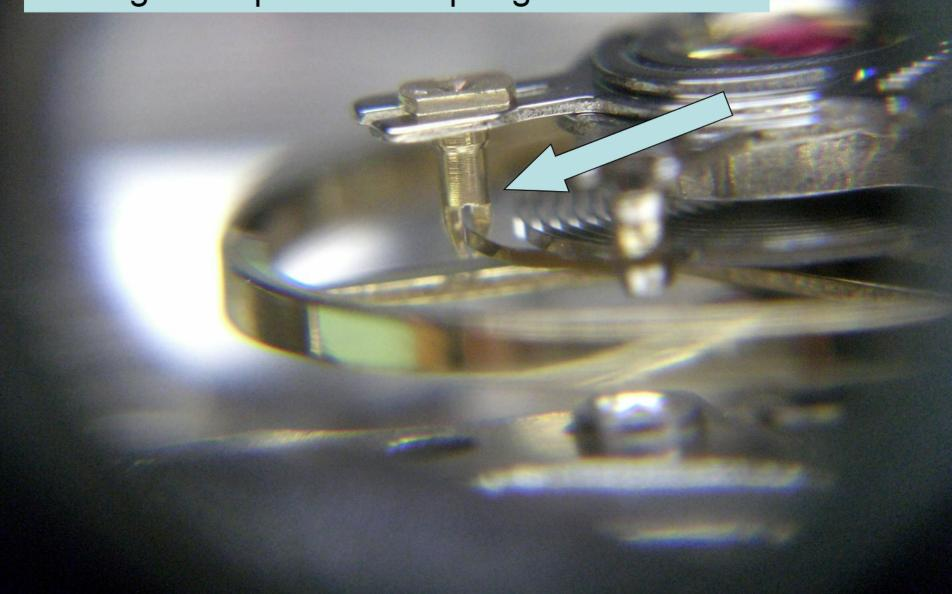
To adjust the spacing at the regulator pins, **slightly** turn the stud block in the direction needed **while viewing** the spacing between the regulator pins and the hairspring.
